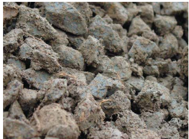
Figure 6. CU-Soil, the structural soil developed at Cornell University in the 1990s. Soil particles within the media are clearly visible and allow soil nutrients and water holding capacity for healthy root growth.
