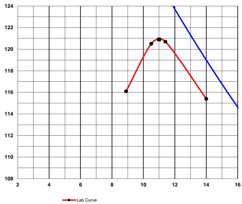
Maximum Dry Unit Weight & Optimum Water Content Zero Air Voids
